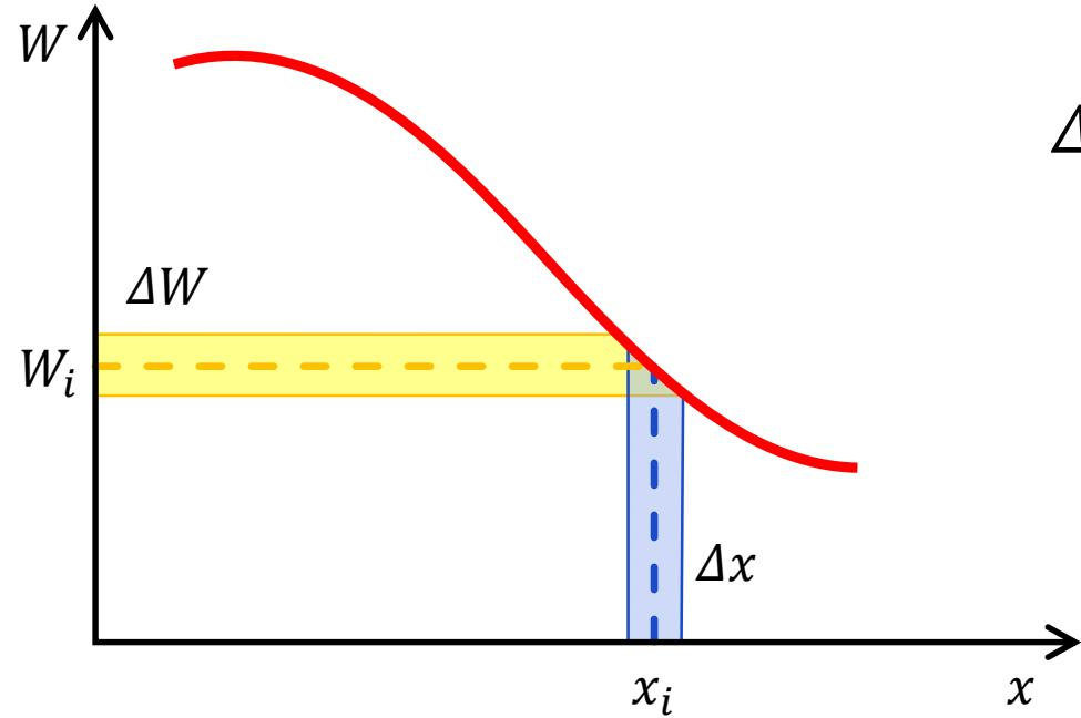
$$\Delta W^2 = \left( \frac{\partial W}{\partial x} \right)^2 \Delta x^2 + \left( \frac{\partial W}{\partial y} \right)^2 \Delta y^2 + \left( \frac{\partial W}{\partial z} \right)^2 \Delta z^2$$
